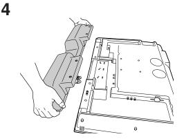
Remove the two speaker plugs from the terminal on the Display.
